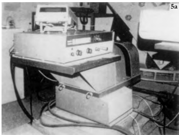
Fig. 5 Elettromagnete E 104B/EPR (Varian) (a, b) Electromagnet E 104B/EPR (Varian) (a, b)
